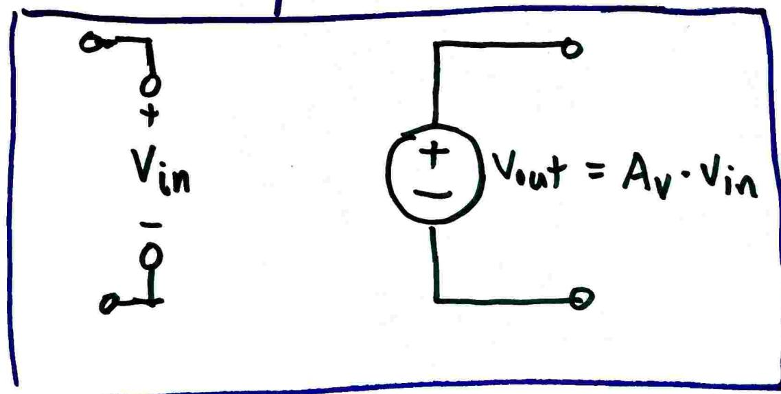
Voltage Controlled Voltage Source
