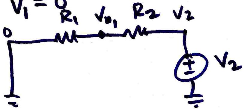
$$V_{n1} = V_2 \cdot \left( \frac{R_1}{R_1 + R_2} \right)$$
