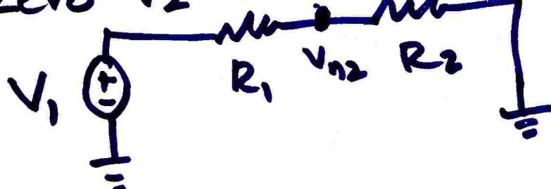
$$V_{n2} = V_1 \cdot \left( \frac{R_2}{R_1 + R_2} \right)$$
