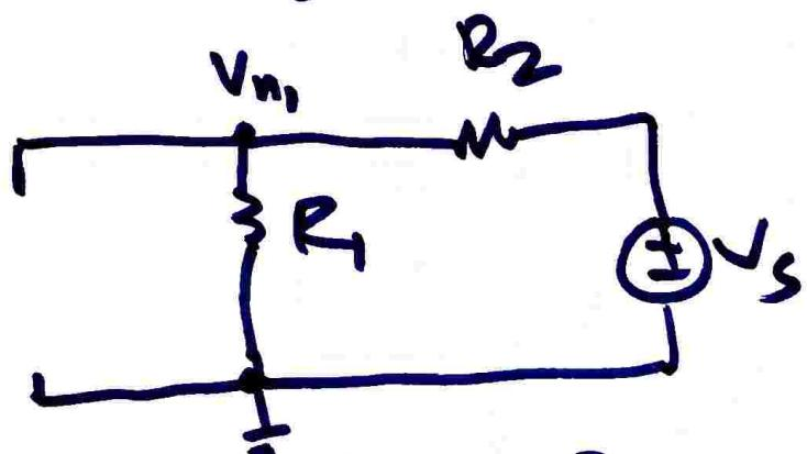
$$V_{m1} = V_s \left( \frac{R_1}{R_1 + R_2} \right)$$
