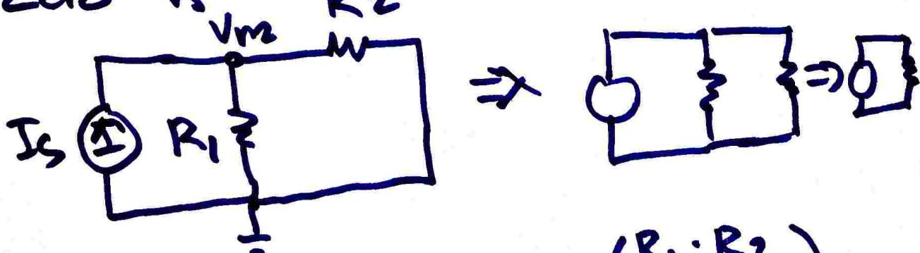
$$V = IR = I_s \cdot R_{eq} = I_s \left( \frac{R_1 \cdot R_2}{R_1 + R_2} \right)$$
