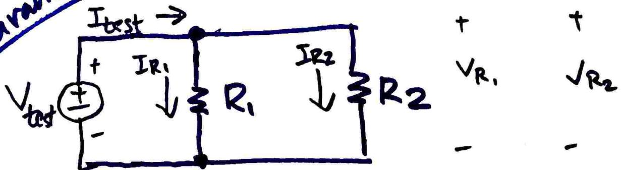
$$I_{\text{test}} = I_{R_1} + I_{R_2}$$
