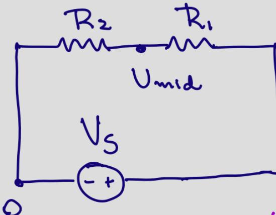
$$U_{mid} = \frac{R_2}{R_2 + R_1} \cdot V_s \quad (\text{Voltage Divider})$$
