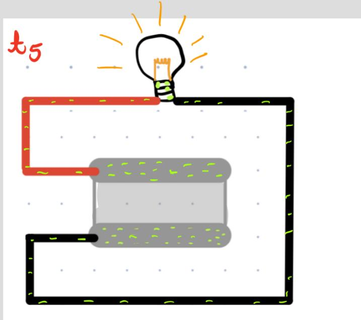
The capacitor will charge a "load" until the charges on the plate are equalized. (No change in  $V$ )
