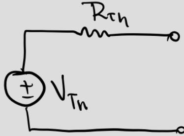
$$R_{Tn} = \frac{V_{test}}{I_{test}} = (R_1 + R_2)$$
