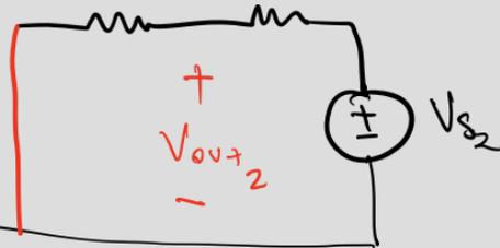
$$V_{out2} = \frac{R_1}{R_1 + R_2} \cdot V_{s2}$$
