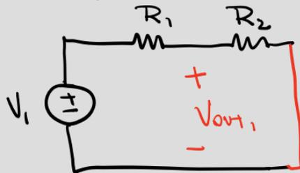
$$V_{out1} = \frac{R_2}{R_1 + R_2} \cdot V_{s1} \quad \text{😊}$$
