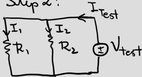
$$I_1 = \frac{V_{test}}{R_1}$$
