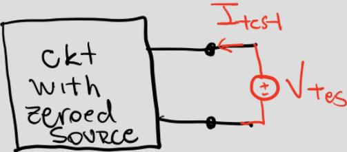
$$R_{Th} = \frac{V_{test}}{I_{test}}$$
