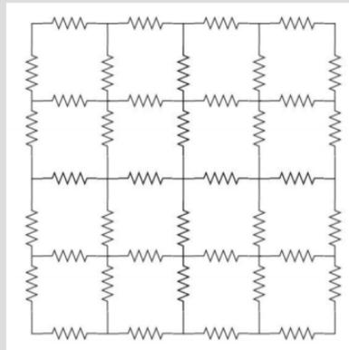
Circuit model for each resistive sheet is a grid of resistors
