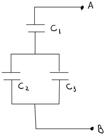
$$C_{eq} = C_1 \parallel (C_2 + C_3)$$
