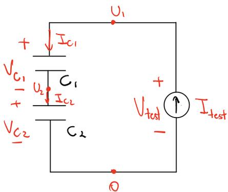
KCL :  $I_{C1} = I_{C2} = I_{test}$
