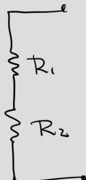
$$\equiv R_{\text{eq}} = R_1 + R_2$$
