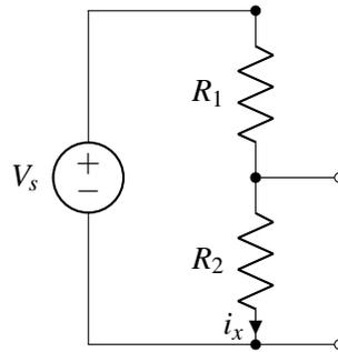
(b) For the circuit below, find the current through  $R_2$ .
