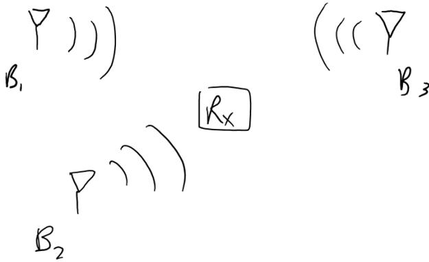
Our goal is to figure out where the receiver is. In order to do that, we need to be able to estimate the distance between the receiver and the beacon transmitters. As we will see, once we have those distances, we can figure out where we are.
