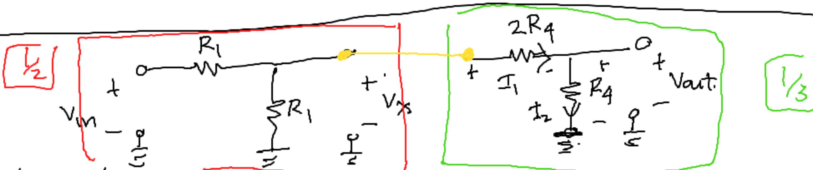
Does  $V_{out} = \frac{1}{6} V_{in}$ ?
