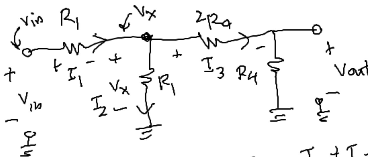
$$V_{\text{out}} = \frac{2R_4}{R_1} V_{\text{in}} - \frac{12R_4}{2+R_1} V_{\text{out}}$$
