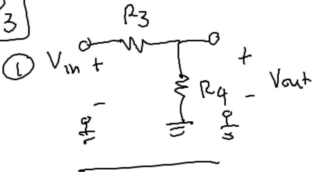
$$V_{out} = \frac{1}{3} V_{in}$$
