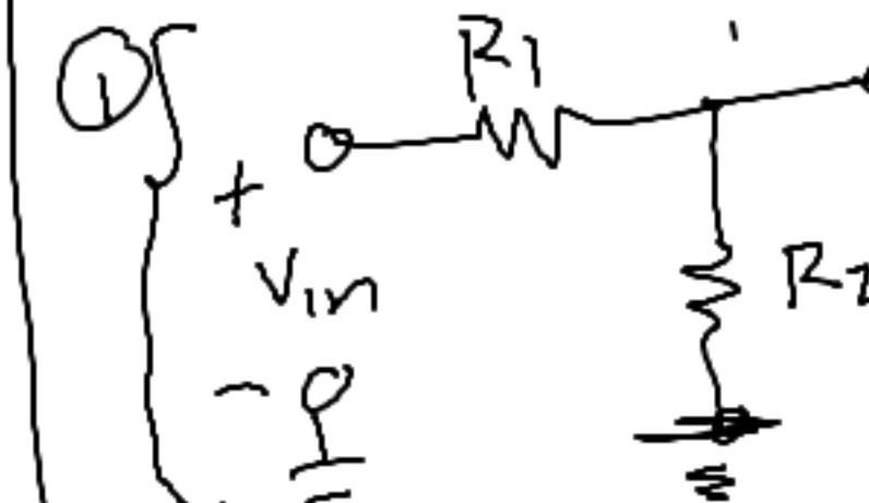
$$\textcircled{2} \quad V_{out} = \frac{R_2}{R_1 + R_2} V_{in}$$
