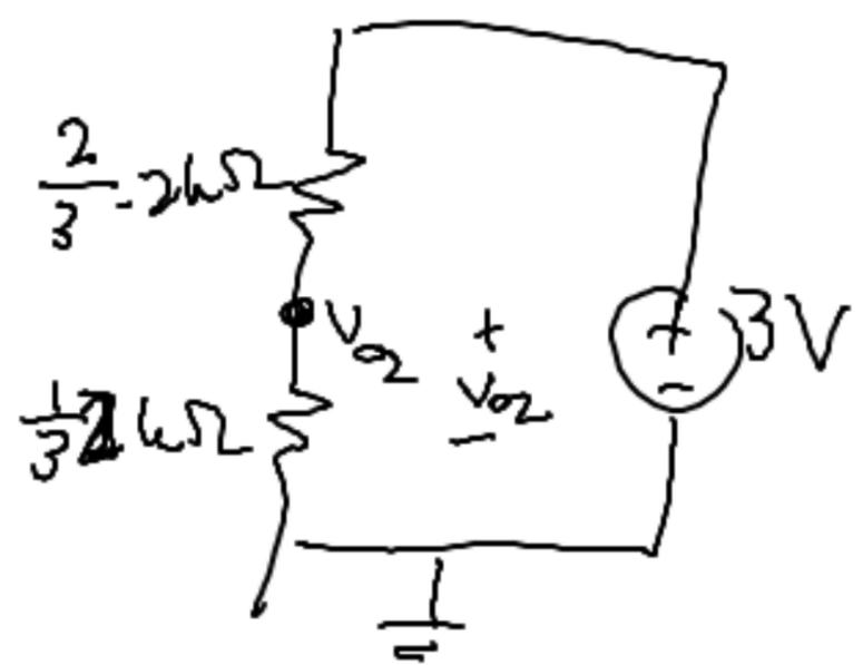
$$V_{02} = \frac{R_{bot}}{R_{bot} + R_{top}} V_S$$
