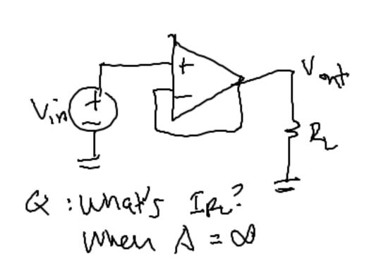
When  $\Delta \neq \infty$ Vant =  $\frac{1}{1+\Delta}$  Vin  $I_{R_L} = \frac{Vant}{1+\Delta} \neq 0$
