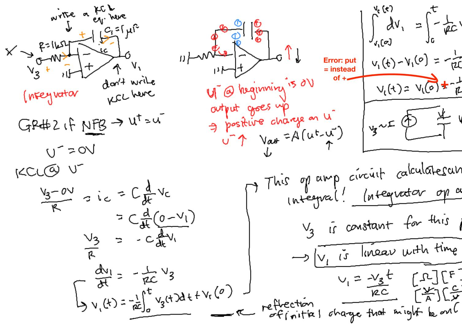
$\int_{v_1(c)}^{t} dv_1 = \int_{c}^{t} \frac{1}{pc} v_3 dt$  $v_{1}(t) - v_{1}(c) = -\frac{1}{2c} \int_{0}^{t} v_{3}(t) dt$  $V_{1}(t) = V_{1}(0) + \frac{1}{RC} \int_{0}^{t} V_{3}(t) dt$ your the Kurt= It This op amp circuit calculates an integral! Integrator op amp V3 is constant for this problem -> [v, is linear with time] Q=CV  $v_1 = -v_3 t [r][F] = \frac{a}{v_1} = c$ NC [茶][乐]-[索][乐] = seconds
