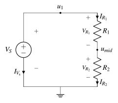
• Step 5: Write KCL equations for all nodes with unknown voltage - in this case, this is just  $u_{mid}$ , since  $u_1 = V_S$ . The current entering that node is  $I_{R_1}$  and the current leaving it is  $I_{R_2}$ . Since these currents must be equal,
