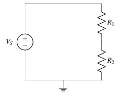
• Step 2: Label the node connected to the voltage supply as  $u_1 (= V_S)$ , since the voltage supply goes between this node and ground.
