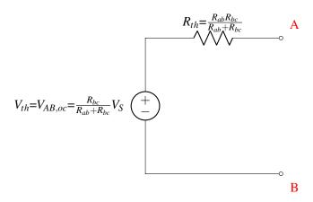
What if we instead chose the upper two nodes (instead of the lower two nodes) as the two terminals (nodes A and B)? We can follow the same procedure to find an equivalent Thevenin circuit from the standpoint of these new nodes,
