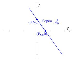
We call the first circuit below, containing a voltage source and a resistor the **Thevenin equivalent circuit**; we call the second circuit, containing a current source and a resistor, the **Norton equivalent circuit**. Once we simplify the original circuit to one of the above, we can easily figure out  $V_{out}$  no matter what resistor it is connected to on the right. In fact, we can convert **any** circuit into any one of these equivalent forms.
