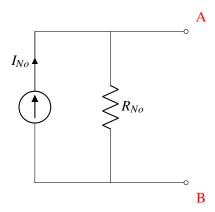
What about solving for the Norton equivalent circuit? First, note that  $R_{No}$  is equal to  $R_{Th}$ , since the slope of the IV curve is the same. Now, instead of looking at the V axis intercept, we find the intersection with the I-axis: At the intersection with the I-axis, the voltage drop between A and B is zero, which is equivalent to placing a wire between A and B (i.e. shorting A and B). We denote the current through the wire be  $I_{SC}$ .
