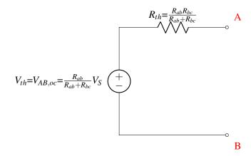
This is not the same result! In this case, the Thevenin voltages in the two circuits are different. This example shows how different pairs of nodes in the same circuit result in different equivalent circuits. In general, there is no guarantee that circuits will behave in the same way from the standpoint of different pairs of nodes.
