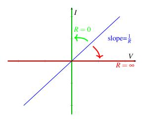
We know that the slope of the line is equal to  $\frac{1}{R}$ . What happens in the limit where R trends towards infinity? Then the line becomes the x-axis, which corresponds to an open circuit as we've seen earlier. Now what happens in the limit where R trends towards zero? The line becomes the y-axis, which corresponds to a wire.
