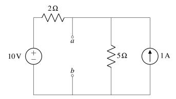
8. For the same circuit above, what is the equivalent Thevenin resistance between the nodes a and b?
