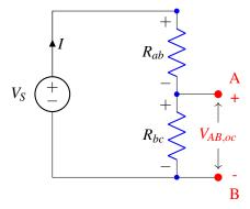
Note that the same current flows through the two resistors. In addition, the voltage drop over the two resistors sums to  $V_s$ , so we can write  $V_{Rab} = V_s - V_{AB,oc}$ . Therefore, using Ohm's Law:
