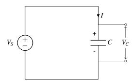
We know that initially, charges are going to build up on the two plates — positive charges on the top plate and negative charges on the bottom plate. Once enough charge has been stored, the voltage across the capacitor becomes  $V_C = V_S$ ; because the voltage can no longer increase past this point, the current *I* flowing through the circuit becomes zero.
