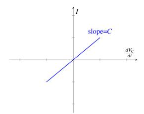
An important implication of this is that **current is only flowing through the capacitor if the voltage across the capacitor is changing with time.** If the voltage is no longer changing, then the current through the capacitor will equal 0.
