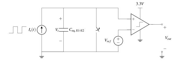
First, note that the voltage over the capacitor  $V_c$  is equal to the voltage at the positive terminal of the comparator ( $U_+ = V_c$ ). The negative terminal of the comparator is connected to  $V_{ref}$  so  $U_- = V_{ref}$ . Using the equations for a comparator, we can write
