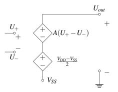
This circuit includes two voltage-controlled voltage sources. (Note that the dependent voltage sources in the schematic above are referenced to  $V_{SS}$ , not ground.) The bottom voltage source adds the voltage  $\frac{V_{DD}-V_{SS}}{2}$  so that when  $U_+ = U_-$ , the output voltage is the midpoint between  $V_{DD}$  and  $V_{SS}$ . The top source creates a voltage  $A(U_+ - U_-)$ , which amplifies the difference between the two input terminals.
