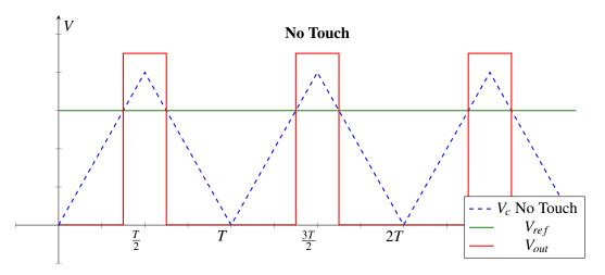
Every period of the current source cycle, we can measure if there is a finger touching this pixel. Later in this course, we will learn how to build a periodic current source like the one needed in this design — after that you will be ready to completely build your own capacitive touchscreen!
