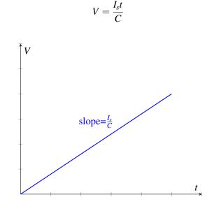
where t is the time passed since we started charging the capacitor. If we measure the voltage at a known time t, we can solve for the capacitance. However, as time continues to pass, the voltage across the capacitor (and also the charge stored on the capacitor) will grow to infinity. It is very challenging to build an ideal current source that works over this large range of voltages, so our model quickly becomes unrealistic.
