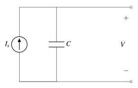
If the capacitor starts off at t = 0 with no voltage across it, we find that V is:
