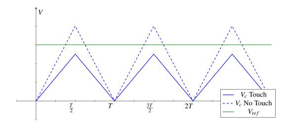
When there is a finger present,  $V_c$  is always less than  $V_{ref}$  so the output voltage is 0:
