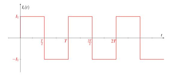
What does the voltage V look like with this current source? Let's assume that the capacitor is initially uncharged (ie. Q = 0). Since Q = CV, this means that at time t = 0 the voltage V = 0. (We will revisit this assumption later.)
