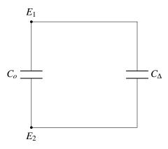
Finally we consider the parallel combination of  $C_o$  and  $C_{\Delta}$  as some equivalent capacitance  $C_{eq, E1-E2} = C_o + C_{\Delta}$ . When the finger is present,  $C_{\Delta} > 0$ , and the equivalent capacitance  $C_{eq, E1-E2}$  will be greater than
