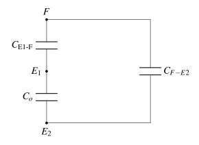
Our touchscreen can only measure things that are between electrodes  $E_1$  and  $E_2$  as it is impractical to physically connect a measuring device to our finger. So, we redraw our circuit as follows:
