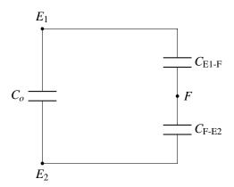
We can further simplify the circuit by replacing the series combination of  $C_{E1-F}$  and  $C_{F-E2}$  by some capacitance  $C_{\Delta}$ . When the finger is present,  $C_{E1-F}$  and  $C_{F-E2}$  have positive capacitance, so we know  $C_{\Delta}$  has some capacitance greater than zero.
