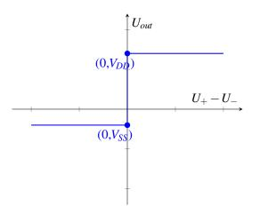
Since A is very large, there is a very sharp transition in the center of the plot. Therefore, when  $U_+ < U_-$  (or equivalently, when  $U_+ - U_- < 0$ ), then  $U_{out}$  equals  $V_{SS}$ . Similarly, when  $U_+ > U_-$ , then  $U_{out}$  equals  $V_{DD}$ . In this case, the op-amp is acting as a comparator since it indicates which voltage ( $U_+$  or  $U_-$ ) is larger, even if the difference between them is very small.
