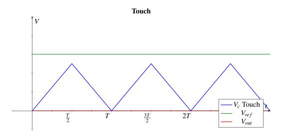
When there is no finger present, then there will be an increase in  $V_{out}$  when  $V_c$  is higher than  $V_{ref}$ :
