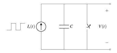
When the switch is closed, it acts as an ideal wire, so the voltage across the capacitor is 0. Since Q = CV, this means that the charge is zero as well, so sometimes we refer to this switch as "discharging" the capacitor.
