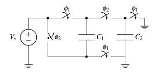
**Step 1:** Label the voltages across all the capacitors. Choose whichever direction (polarity) you want for each capacitor - this means you can mark any one of the plates with the "+" sign, and then you can mark the other plate with the "-" sign. Just make sure you stay consistent with this polarity across phases.
