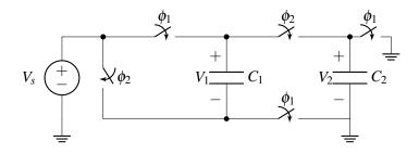
**Step 2:** Draw the equivalent circuit during both phases. For this problem, phase 1:  $\phi_1$  closed,  $\phi_2$  open, and phase 2:  $\phi_1$  open,  $\phi_2$  closed. Also, label all node voltages on the circuit for both phases. No need to try and maintain the same names, since certain nodes of the phase 1 circuit might be merged or split in phase 2.
