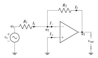
Let's assume that this circuit is in negative feedback so that we can use golden rule #2, after analyzing the circuit we will show how to check if a circuit is indeed in negative feedback.
