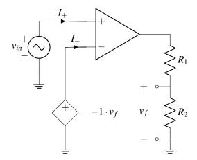
Step 1: Zero out all independent sources. We cannot zero out controlled voltage source  $-1 \cdot v_f$  because this is not an independent voltage source.
