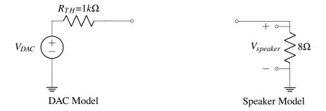
In this example, we'd like  $V_{speaker} = V_{DAC}$ , so that the DAC output is directly played on the speaker. We try connecting the DAC and speaker together directly:
