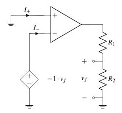
**Step 2: "Dink"**  $v_{out}$ . If we increase  $v_{out}$ ,  $v_f$  increases which then decreases  $v_- = -1 \cdot v_f$ , which then increases  $v_{in} = u_+ - u_-$ , thus  $v_{out}$  increases. The circuit response to the increase in  $v_{out}$  is in the same direction as we "dinked"  $v_{out}$ . So this circuit is not in negative feedback.
