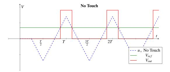
$V_{out}$  has the same structure as when we used an ideal current source! However, since one terminal of our "almost" current source is always 0V, the analysis was slightly different and we had to rethink the circuit architecture. That's why Step 4 (Verification) of the design procedure is so important – we can't assume different circuit blocks will act the same when we connect them.
