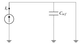
After the button is pressed, the switch is off and can be replaced by an open circuit, and everything functions as it did before.
