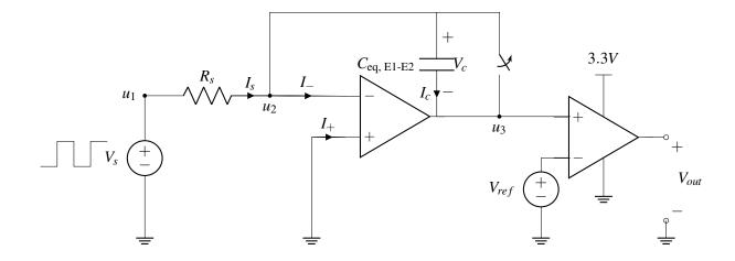
By the second golden rule (applied to the left op-amp),  $u_2 = U_+ = 0V$ . We can use KVL to determine that
