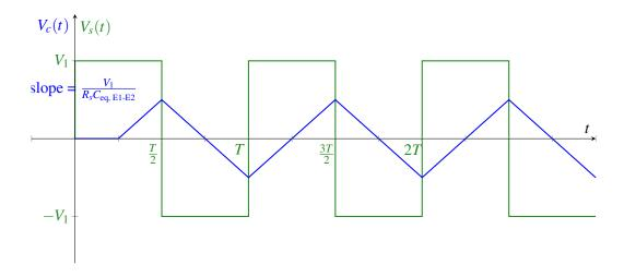
Recalling that  $C_{\text{eq, E1-E2}}$  increases when there is a touch, we can plot  $u_+ = -V_c$  when the finger is present and absent. We'd like to set  $V_{ref}$  halfway between the peak of  $u_+$  with a touch and  $u_+$  without a touch.
