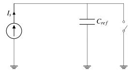
Before the button is pressed, the switch is closed and can be replaced by a wire. In this case, the current from the current source can flow through this wire to ground, eliminating the contradiction that happened before. In addition, when the switch is closed, it connects the top of the capacitor to ground, so the voltage drop over the capacitor remains constant at 0.
