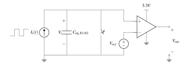
Here, the current source,  $I_s$ , outputs a period square wave that alternates between  $I_1$  and  $-I_1$ . The voltage over the capacitor  $V_c$  increases linearly, with a slope that depends on  $C_{\text{eq, E1-E2}}$ . The switch is opened at  $t = \frac{T}{4}$ .
