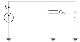
This change in circuit architecture has another important benefit: it guarantees that the initial voltage on the capacitor is 0V. This is important because we used this assumption when setting  $V_{ref}$  in Eq.(3). Without this change, we would not know the initial voltage, and therefore we could not choose  $V_{ref}$  to correctly correspond to 2 sec.
