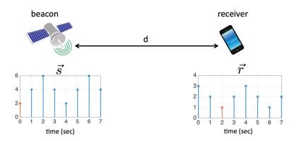
Our goal is to determine this time delay,  $\tau$ . Then we can use the velocity of radio waves (or light, or sound),  $\nu$ , to determine the distance:  $d = \nu \tau$ .
