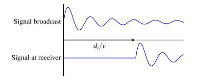
Notice that the received signal is delayed by some amount, due to its travel time. As we discussed earlier, letting  $d_i$  be the distance between the receiver and the beacon, this delay will equal  $d_i/v$ .
