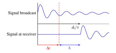
As shown above, the recording begins only after some time  $\Delta t$ . When we perform cross-correlation, we determine that the signal has been delayed by some time  $t_i$  after we began recording. But as shown in the above diagram, the signal has in fact been traveling for a time  $t_i + \Delta t$ , not simply  $t_i$ .
