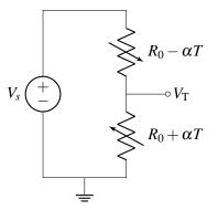
Figure 17: Temperature Sensing Circuit
