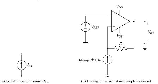
Figure 3: Circuits detailing the transresistance amplifier design, including the background signal Idamage.
