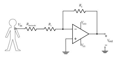
Figure 5: An alternative ECG op-amp circuit.
