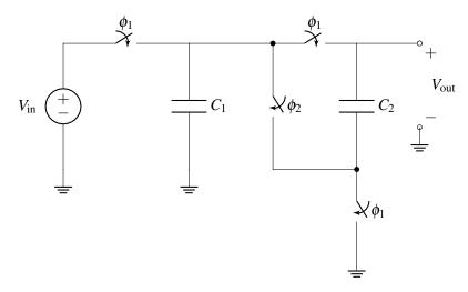
Figure 7: Switch capacitor voltage boosting circuit.
