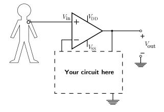
Figure 4: Unfinished ECG amplification circuit.
