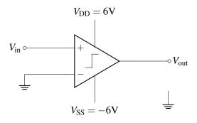
Figure 18: First attempt eye-pad control circuit.
