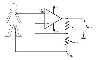
Figure 6: Alternative op-amp ECG topology.
