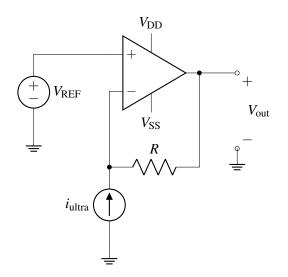
Figure 2: Transresistance sensor circuit
