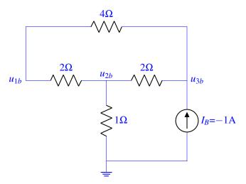
As with part (a), due to symmetry, we can use the results from the case where only the current source  $I_A$  is active. However, since  $I_B$  is "flipped" relative to part (a) – i.e. the value of  $I_B$  is negative – we simply need to scale our answers from part (a) by -1. Taking the symmetry and sign information into account, we arrive at:
