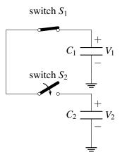
Figure 8.6: Two DRAM cells in parallel. Switch  $S_1$  is closed (can be thought of as a wire), and switch  $S_2$  is closing.
