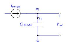
A single KCL equation at node  $u_1$  gives  $I_{switch} = i_1$ , where  $i_1 = \frac{dQ}{dt} = C_{DRAM} \frac{dV_{out}}{dt}$ . We integrate and solve for  $V_{out}(t)$  at t = 1 ms as follows:
