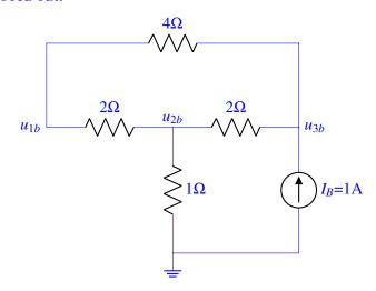
This circuit is very similar to when  $I_B$  is zeroed out, just with the relative positions of the nodes with respect to the active current source modified. So we can observe that:
