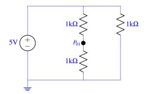
We can therefore solve for the voltage at  $P_{01}$  as a voltage division of 5V:  $P_{01} = 5V \frac{1k\Omega}{1k\Omega+1k\Omega} = 2.5V$ . No other point on the circuit has this voltage. Therefore, yes, we can identify where the touch happened, and we can do so uniquely as there is only one point that exists with this voltage:  $P_{01}$ .
