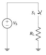
Figure 4.1: Model of resistive load bank in a circuit.
