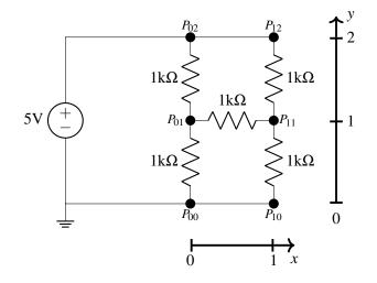
Figure 6.1: A schematic of the H-shaped resistive touchscreen.
