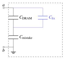
Figure 8.5: Your fabricated DRAM cell with an additional mistake capacitance,  $C_{\text{mistake}}$ , and a capacitance intentionally added to fix the mistake,  $C_{\text{fix}}$ .
