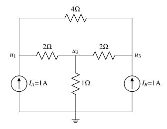
Figure 7.1: Schematic for part (a).
