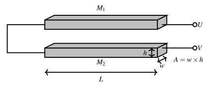
Figure 5.1: Resistive metal bars connected through ideal wires.
