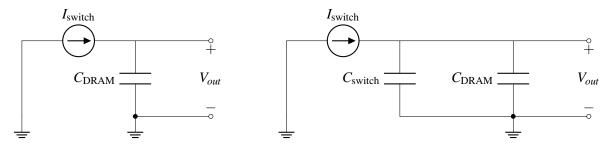
Figure 8.3: Left: Circuit without parasitic capacitance. Right: Circuit with parasitic capacitance.
