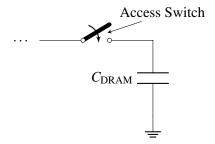
Figure 8.1: A DRAM cell consisting of an access switch and a capacitive storage element, C<sub>DRAM</sub>.
