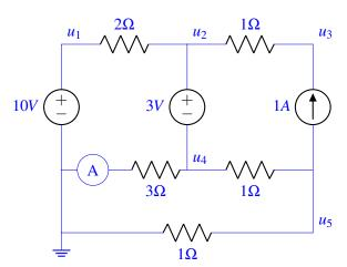
Figure 3.6: Ammeter placement to measure current flowing through the  $3\Omega$  resistor.
