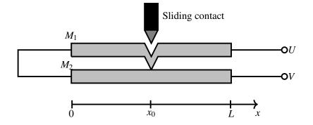
Figure 5.2: Sliding switch making a contact between  $M_1$  and  $M_2$ .
