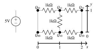
Figure 6.3: Resistor grid for part (d).
