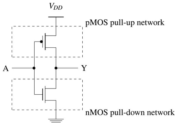
In general, a Boolean-formula circuit has an nMOS *pull-down network* to connect the output to 0 (GND) and a pMOS *pull-up network* to connect the output to 1 ( $V_{DD}$ ). The pull-up and pull-down networks in the inverter example each consist of a single transistor.
