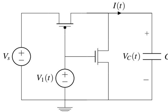
In this circuit, the source of the PMOS transistor is connected to the positive node of  $V_s$  and the source of the NMOS transistor is connected to ground.  $|V_{th}| = 2V$  for both transistors.  $R_p = R_n = 1k\Omega$  for the transistor resistances and  $V_s = 5V$ .  $V_1(t)$  is defined as follows:
