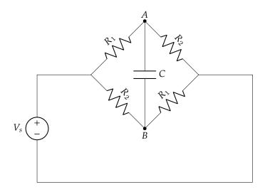
Figure 1: Modified Wheatstone bridge circuit.
