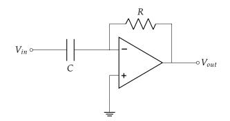
Figure 4: Operational Amplifier with RC elements.
