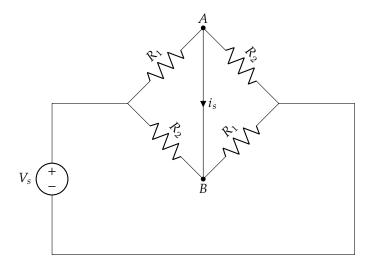
Figure 2: Modified Wheatstone bridge circuit.
