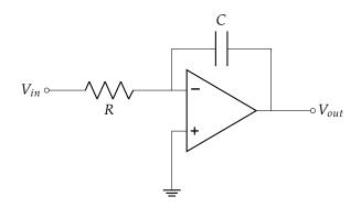
Figure 3: Operational Amplifier with RC elements.
