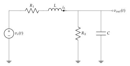
Figure 1: A model for a transmission line.
