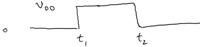
Figure 3.5: Input signal to the first inverter of Figure 3.4
