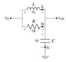
For the RLC filter above, with component values  $R = 1 \text{ k}\Omega$ , C = 10 nF, and  $L = 1 \mu\text{H}$ ,
