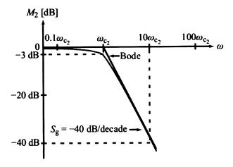
(b) Derive a transfer function that would result in the following bode plot. Hint.  $20\log_{10} 2 = 6$ .
