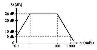
(c) Derive the transfer function and plot the magnitude and phase bode plots for the following. For the
