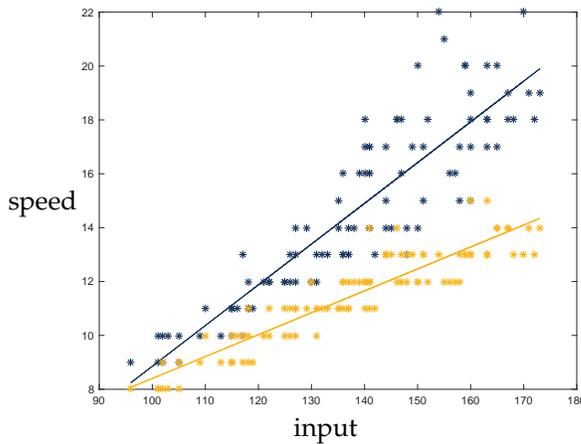
Figure 2: Speed vs. input data points from experiments. The left and right wheels are represented with different colors, and the lines show least squares estimates for each.
