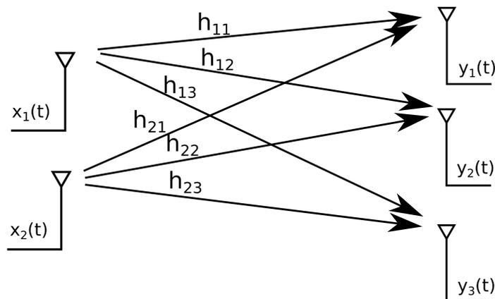
$$\begin{bmatrix} h_{11} & h_{21} \\ h_{12} & h_{22} \\ h_{13} & h_{23} \end{bmatrix} \cdot \begin{bmatrix} x_1(t) \\ x_2(t) \end{bmatrix} = \begin{bmatrix} y_1(t) \\ y_2(t) \\ y_3(t) \end{bmatrix}$$
