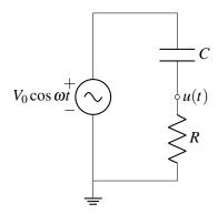
We are interested in knowing how the voltage u(t) varies over time. Recall that we proved the voltage divider equation in the context of DC circuit analysis. However, that proof carries over to the phasor domain in a straightforward manner. Thus, the phasor  $\widetilde{u}$  representing the voltage u(t) can be represented in terms of the phasor  $\widetilde{V}$  representing the supply voltage as follows:
