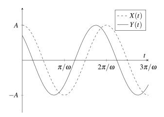
Here,  $\phi$  represents the *phase shift* of Y with respect to X. As can be seen, a positive phase shift moves the function to the left by that amount. In particular, notice that the sine and cosine functions are really the same sinusoid, with each just the other after a  $\pi/2$  radian phase shift in the appropriate direction.
