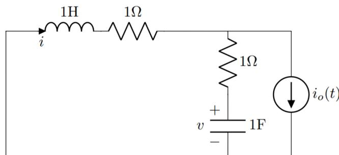
Consider the circuit above with the inductor current  $i$  and capacitor voltage  $v$  as state variables and with the independent current source  $i_o$  as input.
