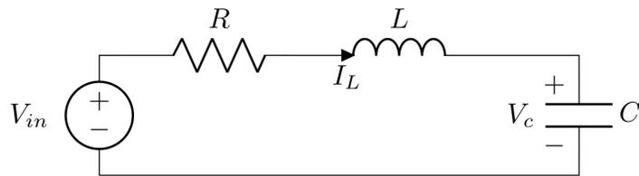
Let the circuit's dynamics be modeled by the state space equation  $\frac{d}{dt}\vec{x}(t) = \mathbf{A}\vec{x}(t) + \vec{b}u(t)$ . What is a necessary condition for the eigenvectors of  $\mathbf{A}$  to have non-zero imaginary components?
