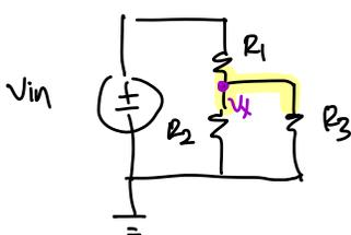
**Step 1:** Pick a node to perform KCL on. Pick a node that has the most # of elements connected to it + what we're interested in
