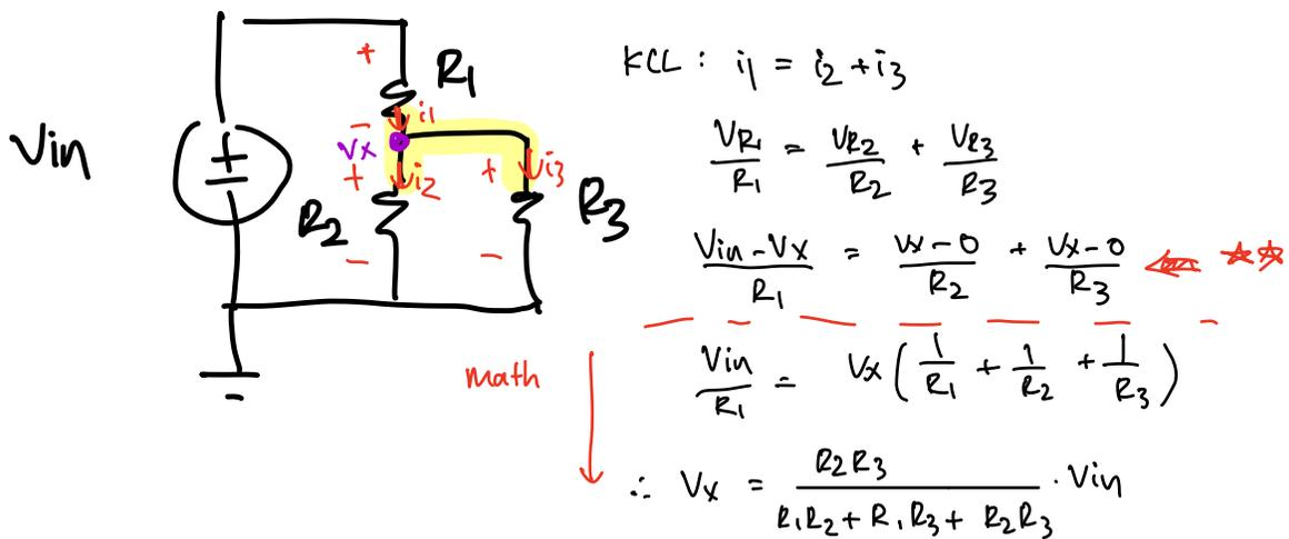
(b) Alternatively, you can realize that  $R_2 \parallel R_3$
