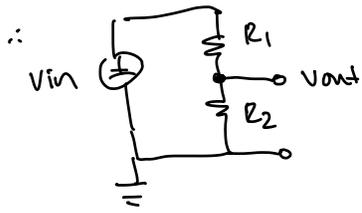
$$V_{out} = \frac{R_2}{R_1 + R_2} \cdot V_{in}$$
