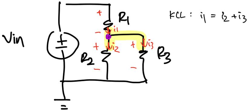
Step 3: Convert your KCL equation into V-R relationships or capacitor relationships, etc.  $V = IR$ ,  $i_C = C \frac{dV_C}{dt}$
