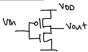
if  $V_{IN} = V_{DD}$ ,  $V_{OUT} = 0V$
