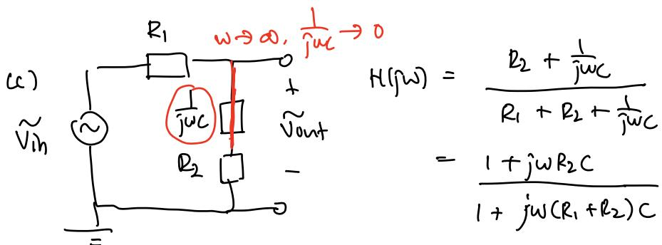
$$\left. \begin{array}{l} \omega \rightarrow 0, |H(j\omega)| \rightarrow 1 \\ \omega \rightarrow \infty, |H(j\omega)| \rightarrow \frac{R_2}{R_1 + R_2} \end{array} \right\} \text{No name for this filter}$$
