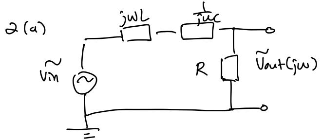
$$H(j\omega) = \frac{R}{R + j\omega L + \frac{1}{j\omega C}} = \frac{R}{R + j(\omega L - \frac{1}{\omega C})}$$
