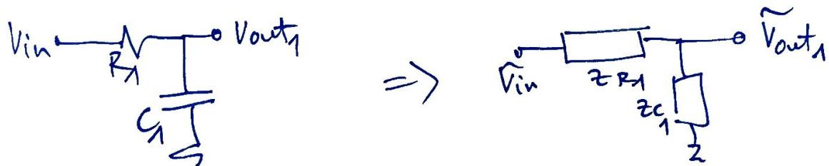
$$H_{LP}(j\omega) = \frac{\tilde{V}_{out_1}}{\tilde{V}_{in}} = \frac{1}{1 + j \frac{\omega}{\omega_{OLP}}} , \quad \omega_{OLP} = \frac{1}{R_1 C_1}$$
