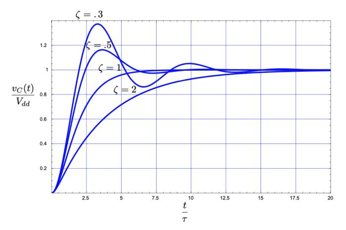
$\zeta < 1$  Underdamped  $\zeta = 1$  Critically Damped  $\zeta > 1$  Overdamped
