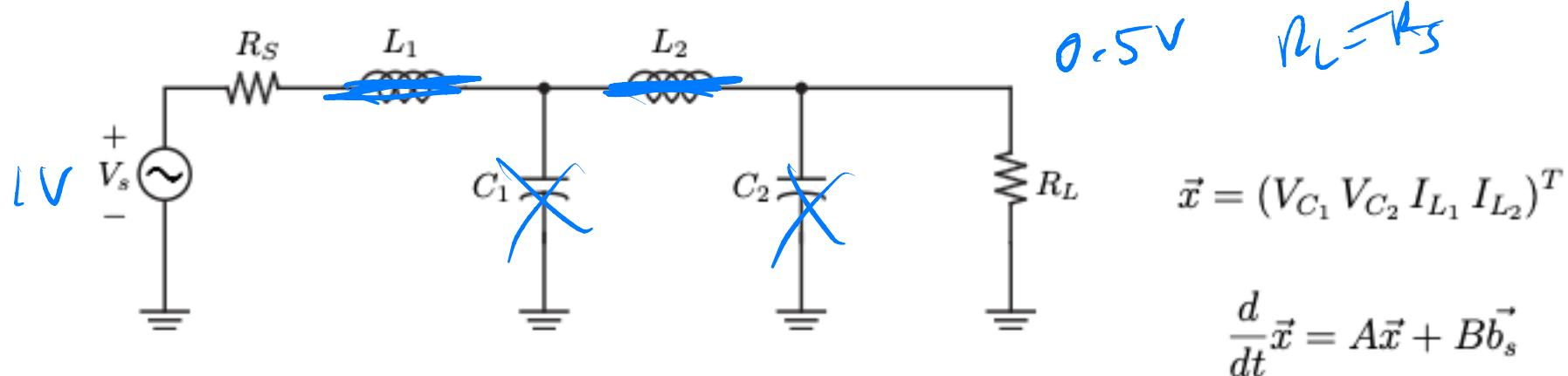
$$A = \begin{pmatrix} 0 & 0 & 1/C_1 & -1/C_1 \\ 0 & -1/R_L C_2 & 0 & 1/C_2 \\ -1/L_1 & 0 & -R_S/L_1 & 0 \\ 1/L_2 & -1/L_2 & 0 & 0 \end{pmatrix}$$
