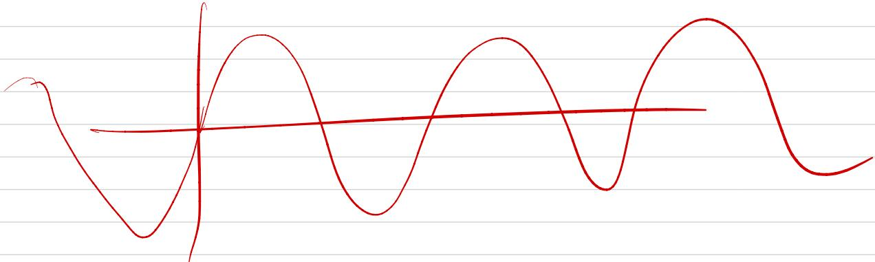
$$v(t) = V_0 \sin(\omega t + \phi)$$
