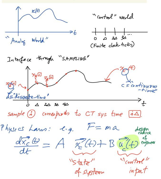
var. you "Care about" ox: state "variable for control system e-g. (i) inductor current, capacitor voltage, etc. in RLC arcusts (ii) position (x14,2), velocity (xx, vy, vz), acceleration (ax, ay, az) etc. in automobile/arroraft combol eys., etc. n: "control" vanable for control system e.q (i) thrust power in aircraft (1) throttle poston in cruise control (iii) independent Voltage or convent Source in RLC circuits. Note: RH and WH can have defeat Note: (x(t)) un.
