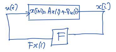
Subst: u[i]= Fa[i] in @ 元(i+1)=(A+BF) 元(i) + e(i) ACL 'closed-loop systen' Q Can we design F s.t. e-vals. of Acc = A +BF ave inside the whit circle (u.c.). het's try some eramples:  $2x \perp (SCALAR) = (2)x(i) + n(i)$ > unstable without fredbork u(i) = f x(i)Clused-loop,' 2(i+1)= (2+4) 2(i) For stability, we want ]2+fl<1 If we want an e-val @ 20 => 2+1=20 14=2-2)
