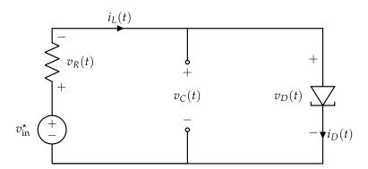
We can linearize this new, simplified system to analyze small perturbations to  $v_C$ ,  $i_L$ ,  $v_{\rm in}$  from the equilibrium states  $v_C^\star$ ,  $i_L^\star$ ,  $v_{\rm in}^\star$ .
