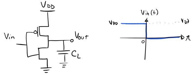
a) If  $v_{in}(t)$  is as plotted above, please provide a differential equation in  $v_{out}(t)$ . (5 points) **Solution:**
