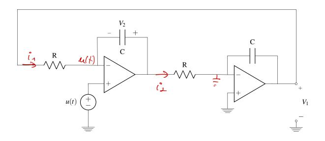
(a) Write a state space model  $\frac{d\vec{x}(t)}{dt} = A\vec{x}(t) + Bu(t)$  with  $\vec{x}(t) = \begin{bmatrix} V_1(t) \\ V_2(t) \end{bmatrix}$ . You can assume the golden rules of op-amps apply here.
