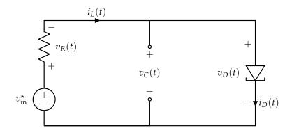
We can linearize this new, simplified system to analyze small perturbations to  $v_C$ ,  $i_L$ ,  $v_{in}$  from the equilibrium states  $v_C^*$ ,  $i_L^*$ ,  $v_{in}^*$ .
