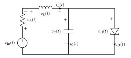
Using KVL and KCL, and the fact that  $i_D(t) = g(v_D(t))$ , we get the state model
