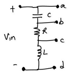
a) (2.5 points) Across which two output terminals would the voltage transfer function look like a low pass filter with respect to  $V_{\rm in}$ ?
