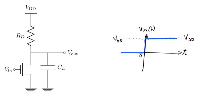
If  $v_{in}(t)$  is as plotted above, please provide a differential equation in  $v_{out}(t)$ . (5 points)
