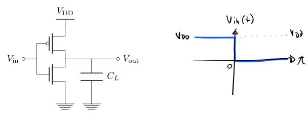
a) If  $v_{in}(t)$  is as plotted above, please provide a differential equation in  $v_{out}(t)$ . (5 points)
