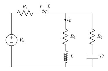
a) Provide a symbolic equation in one variable that can be solved to determine  $v_c(t)$  for  $t \ge 0$ .
