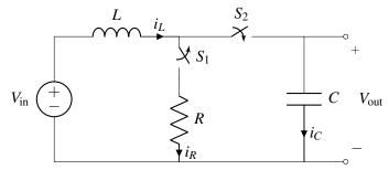
At t < 0,  $S_1$  is on (short-circuited), and  $S_2$  is off (open-circuited). At  $t \ge 0$ ,  $S_1$  is off (open-circuited), and  $S_2$  is on (short-circuited).
