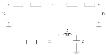
In this problem, we will examine the equivalent impedance of such a structure. As a reminder, the equivalent impedance  $\tilde{Z}_{eq}$  of a circuit with some phasor voltage  $\tilde{V}_{test}$  across it and some phasor current  $\tilde{I}_{test}$  flowing through it is  $\tilde{Z}_{eq} = \frac{\tilde{V}_{test}}{\tilde{I}_{test}}$ .
