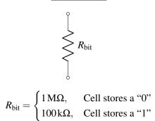
For the rest of this problem, consider the circuit (which is associated with reading out an R-RAM cell) shown below:
