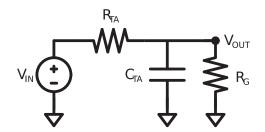
i) Write the fully factored transfer function,  $H(j\omega)$ , in terms of the above variables for our model of the transatlantic cable.
