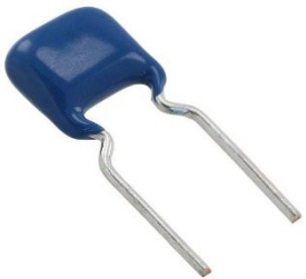
0.1 \mu F \pm 20% 50V Ceramic Capacitor Z5U Radial
