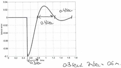
Measured step response (as function of time) on a 10 cm step at 2 m/sec using P+D controller is given as shown above.
